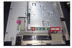
lift up the main bracket and then disconnect the two EDP cables away from the connector of the panel, then take away the main bracket and put it aside.
