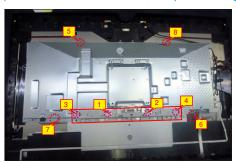
Disconnect the DMIC wire away from the connector of the main board, then lift up and take away the middle S16 frame with front bezel.
