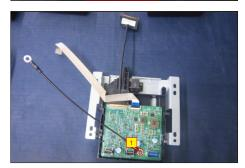
Tear off 2pcs tape, then disconnect the speakers' wire from the connector of the board. Use a Philipshead screwdriver to remove 8pcs screws for unlocking the two speakers, then remove the two speakers from the hooks of the middle frame.
