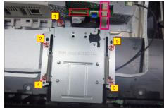
Tear off 2pcs tapes, then disassemble the USB hub cover away from the USB unit. Use a Philips-head screwdriver to remove 1pcs screws for unlocking the USB unit and wire with the bracket, then release the USB board away from the bracket.
