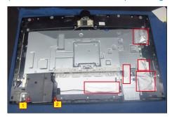
Tear off 1pcs mylar tape, then use a Philips-head screwdriver to remove 5pcs screw for unlocking the wire and USB unit with the bracket and middle frame, then disconnect USB wires and remove the USB unit. (No.1 screw size=M3x6, Torque=5±1kgfxcm;
