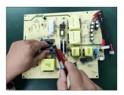
S25-3 Cut into the bottom of bulk cap. and pullit up carefully.
