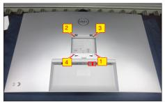
Tear off screen protector, then wedge your fingers between rear cover and the middle bezel on the corners of the top side of the monitor to release the rear cover, then use one hand to press the middle bezel, the other hand to pull up the rear cover in order of arrow preference for unlocking the rear cover.
