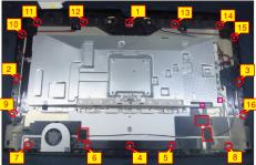
Use the screwdriver to remove 4pcs screws for unlocking the main bracket with the panel. Use a Philips-head screwdriver to remove 4pcs screws for unlocking the bracket cover, and then remove the bracket cover and put it aside.
